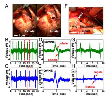
**Fig. 4.** In vivo evaluation of PZT MEHs on the lung and diaphragm. (*A*) Photograph of a PZT MEH cointegrated with a microbattery and rectifier, mounted on the bovine lung. Voltage as a function of time for such devices on the bovine (*B*) and ovine (*C*) lung. *D* and *E* show plots corresponding to the regions indicated by the red dashed boxes in *B* and *C*, respectively. (*F*) Photograph of a PZT MEH on the bovine (*G*) and ovine (*H*) diaphragm.
